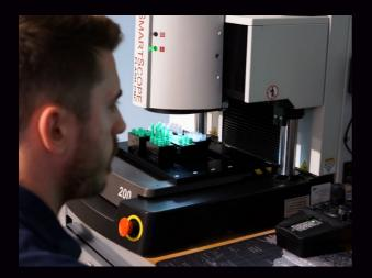
Apacor invested in a <u>SmartScope CNC 200</u> multi-sensor metrology machine from OGP UK to allow them to guarantee accurate, reliable and consistent quality of their components, using the most advanced multi-sensor technology available.
