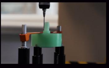
Investing in a multi-sensor metrology system from OGP UK has allowed Dalau to enhance their manufacturing processes and upgrade their old machines to the latest technologies. Dalau is now able to ensure speed, accuracy and traceability when measuring micro and complex components.
