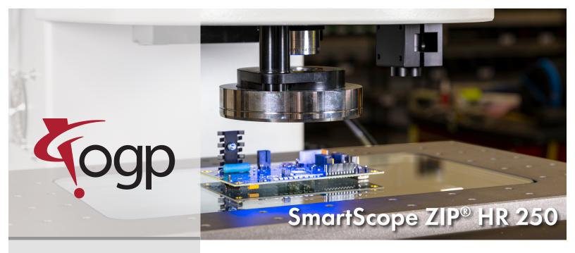
SmartScope ZIP HR 250 benchtop multisensor measurement systems offer versatile optics – a wide field objective lens, digital / optical zoom, and 5-megapixel monochrome digital camera provide a distortion-free image at low zoom, with high resolution at high zoom.
