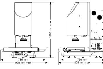
System Weight: 165 kg Shipped Weight: 275 kg
