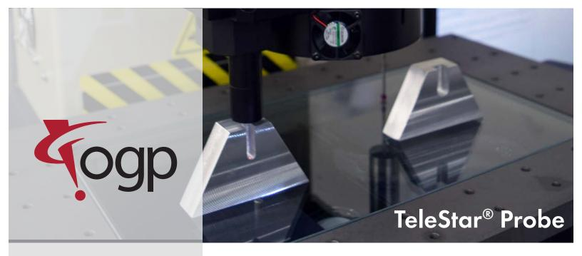
**TeleStar Probe** is a self-contained, off-axis, interferometric range sensor for surface contour measurement. TeleStar Probe offers sub-micron resolution, while scanning either specular or diffuse surfaces. Spot size as small as 5  $\mu$ m for measuring miniature features. The TeleStar Probe offers:
