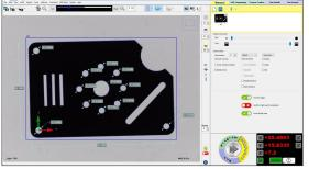
Measure-X software provides users with a simple, powerful interface for instant 2D measurement and auto program generation. The software also utilizes powerful GD&T based algorithms and point and click feature identification to easily program a wide variety of parts. Virtual chart gaging, profile analysis tools and integrated reporting allow for quick and easy output of measurements.
