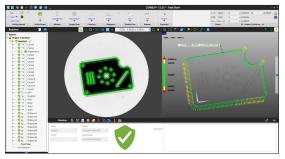
ZONE3 uses innovative features to automatically generate measurement routines resulting in faster programming and run times. Parallel Processing combined with intelligent routine Optimization can be used to measure as many features as can be seen simultaneously
