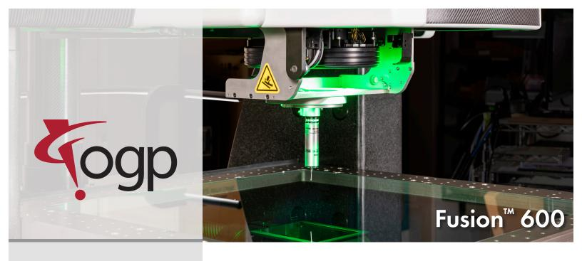
**Fusion 600** is a high-speed, multisensor measurement system with 3D capability that combines an exceptional large field-of-view (LFOV) optical system with multisensor flexibility to form a uniquely productive metrology system. Fusion 600 offers:
