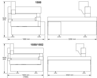
CNC 1500 System Weight: 2590 kg Shipping Weight: 3000 kg
